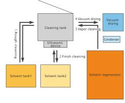
Once the components are loaded into the tank, the entire process is operated automatically, including the replacement of the cleaning solvent. After rough and finish cleaning is completed, the components are rinsed by vapor. The components are then moved onto the vacuum drying process.
