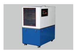
The multi-stage hot air circulation vaporizer is attached or built-in to the cleaning system. Drainage from the cleaning system can be greatly reduced through vaporizing and condensing. If aqueous systems are equipped with one of these, the cleaning chemistry can be recycled when it is moved on to the next tank, meaning a reduction of chemistry filling. Rinsing performance is improved because water can be supplied to the rinsing tank continuously.
